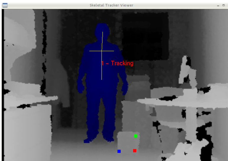
Figure 3. Snapshot of the depth camera tracking display. Four landmarks are automatically detected on the user body: right shoulder, left shoulder, head center and hip center. The three color dots are the user-selected landmarks that define the patient reference system in the posterior-anterior and caudal-cranial directions.
